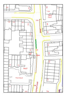
• The junction of Chichester Road with Copnor Road is extended due to the built-out footway to the north. Therefore vehicles and cyclists wait at the junction past the position of the proposed kerbside parking to the south. Currently, cyclists travelling northbound on Copnor Road have to pull out to meet the extended kerbline at this junction: parked vehicles would mean cyclists already taking the direct line northwards without having to pull into the path of traffic.
